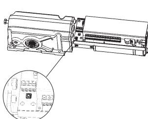
After completion of the mechanical installation and prior to adjusting the parameters, always initiate a calibration run by pressing and holding the pushbutton for 3 flashes of the red LED. This will insure proper door operation by calibrating the unit to the installation conditions.
