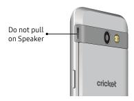
**Warning**: Do not bend or twist the back cover excessively. Using excessive force on the cover during removal or installation of an internal component can cause the material to break.
