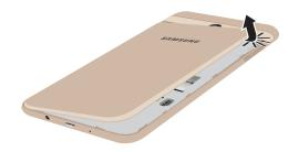
**Caution**: When removing the back cover, use the slot next to the Volume key to gently lift the cover off. Pulling on the Speaker (located next to the Power button) may cause damage.
