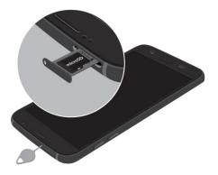
3. Slide the SIM card/Memory card tray back into the slot.
