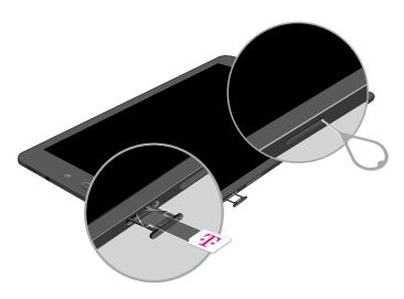
3. Slide the SIM card tray back into the slot.
