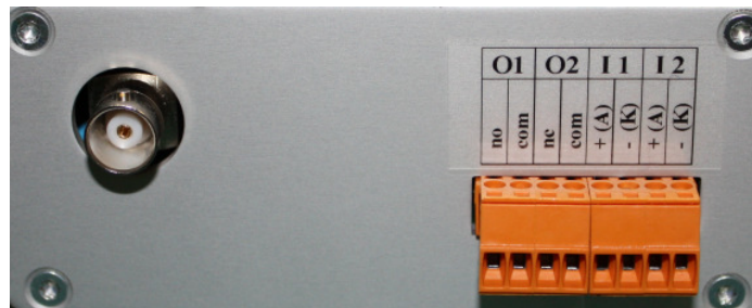
Inputs/outputs of the SIR-2720 13.56 MHz Mid-Range Reader System
