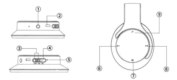
AUX Input Port/Built-in Reset button
