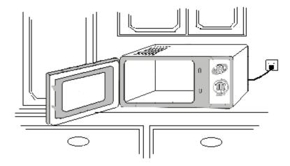
A minimum clearance of 7.5 cm is required between the oven and any adjacent wall. One side must be open.
