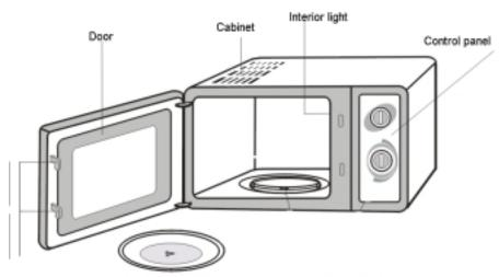
Safey interlock system: Shuts off oven power if door is opened during operation
