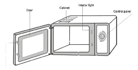
Safey interlock system: Shuts off oven power if door is opened during operation
