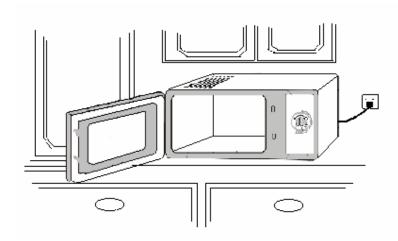
A minimum clearance of 7.5 cm is required between the oven and any adjacent wall. One side must be open.
