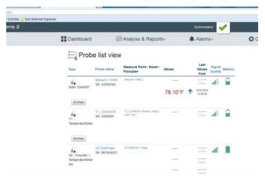
➤ Click name of probe and enter probe detailed information page which show detailed measurement status of each channel. Click "configuration", can enter configuration page to modify configuration of probe.
