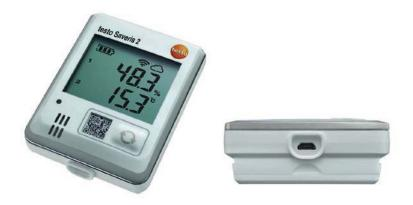
Saveris T2 can support two channel external temperature probe, can continuously measure and record surrounding temperature and transfer to cloud website. Saveris T2 passed EN12830 approval, can use in food industrial surrounding measurement and monitor.
