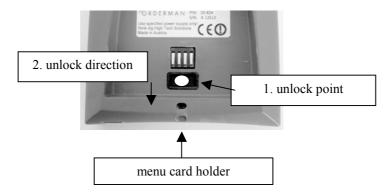
With the end of the entry pen of your ORDERMAN DON touch pen you have to press on to the unlock point. With a simultaneous motion in the unlock-direction, the menu card holder comes out of the housing and can be taken out of the unit. After this, the menu card can be slipped out.
