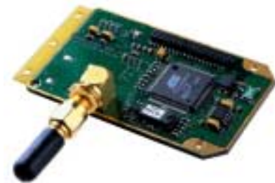
Picture 1 - Stub antenna
