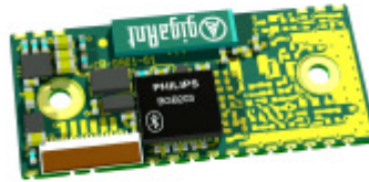
Picture 2: CB-OEMSPA311i-07 OEM Serial Port Adapter short range with internal antenna and a flexfilm connector
