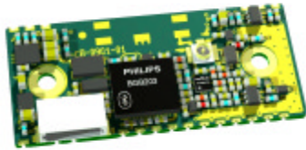
Picture 1: CB-OEMSPA331x-06 OEM Serial Port Adapter long range with external antenna and a JST 6-pol connector
