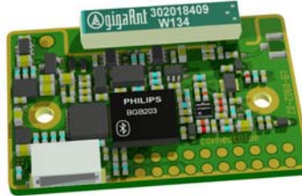
Picture 2: CB-OEMSPA332i-06 OEM Serial Port Adapter long range with internal antenna and JST connector
