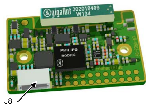
Picture 7: JST 6-pol connector, J8.
