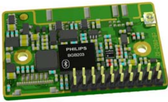
Picture 1: CB-OEMSPA332x-02 OEM Serial Port Adapter long range with external antenna and 2mm pin connector
