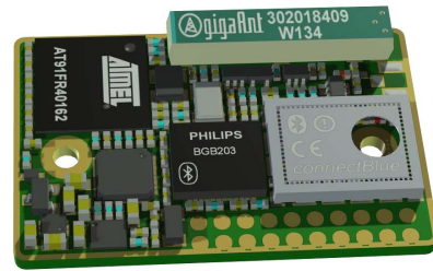
Picture 2: CB-OEMSPA333i-04 OEM Serial Port Adapter long range with internal antenna and no connectors
