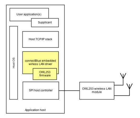
The host needs to be able to hold the target firmware since targets does not have on-board non-volatile memory. At startup, and at every reset or power cycle, the host driver will download firmware binaries to target before any wireless LAN operations can begin.
