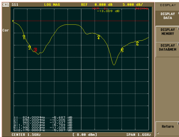
Figure 15: |S_{11}| sample measurement of a penta-band antenna that covers in a small form factor the 4 bands (850 MHz, 900 MHz, 1800 MHz and 1900 MHz)
