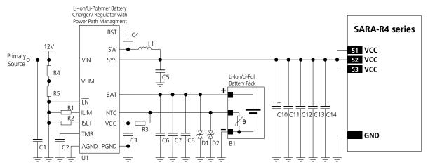
Figure 16: Li-Ion (or Li-Polymer) battery charging and power path management application circuit
