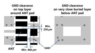
Figure 19: GND keep-out area on top layer around ANT pad and on very close buried layer below ANT pad
