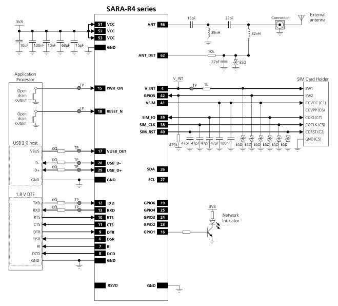
Figure 40: Example of schematic diagram to integrate a SARA-R4 module using all available interfaces
