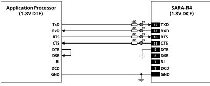
Figure 31: UART interface application circuit with partial V.24 link (5-wire) in the DTE/DCE serial communication (1.8V DTE)
