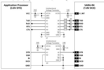
Figure 30: UART interface application circuit with partial V.24 link (6-wire) in DTE/DCE serial communication (3.0 V DTE)
