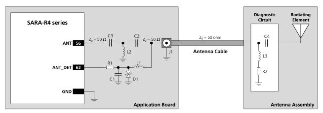
Figure 23: Suggested schematic for antenna detection circuit on application board and diagnostic circuit on antenna assembly
