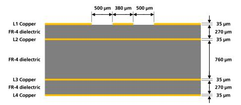
Figure 20: Example of 50  $\Omega$  coplanar waveguide transmission line design for the described 4-layer board layup
