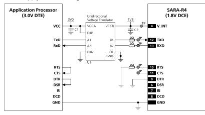
Figure 34: UART interface application circuit with partial V.24 link (3-wire) in DTE/DCE serial communication (3.0 V DTE)
