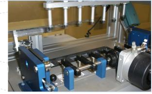
Figure 42: Automatic test equipment for module tests
