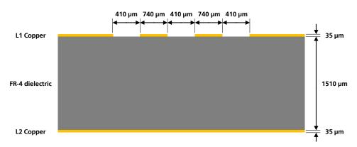
Figure 37: Example of USB line design, with  $Z_0$  close to 90  $\Omega$  and  $Z_{cM}$  close to 30  $\Omega$ , for the described 2-layer board layup
