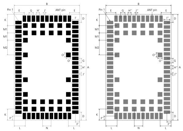
Figure 39: SARA-R4 series modules suggested footprint and paste mask (application board top view)
