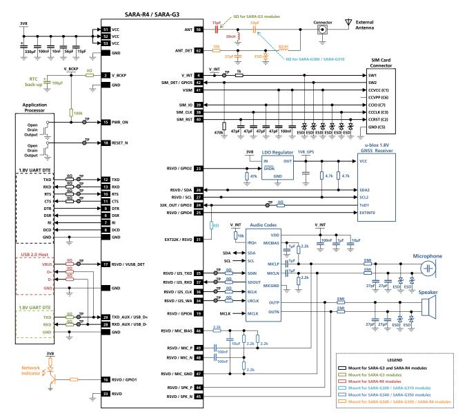
Figure 46: Example of complete schematic diagram to integrate SARA-R4 modules and SARA-G3 modules on the same application board, using all the available interfaces / functions of the modules
