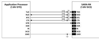
Figure 29: UART interface application circuit with partial V.24 link (6-wire) in the DTE/DCE serial communication (1.8 V DTE)
