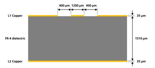
Figure 21: Example of 50  $\Omega$  coplanar waveguide transmission line design for the described 2-layer board layup
