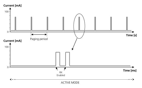
Figure 4: VCC current consumption profile with power saving disabled and module registered with the network: active-mode is always held and the receiver is periodically activated to monitor the paging channel for paging block reception
