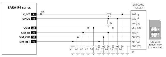
Figure 26: Application circuit for the connection to a single removable SIM card, with SIM detection implemented
