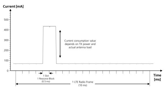
Figure 3: VCC current consumption profile versus time during LTE Cat M1 half duplex connection
