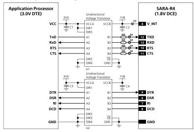
Figure 28: UART interface application circuit with complete V.24 link in DTE/DCE serial communication (3.0 V DTE)
