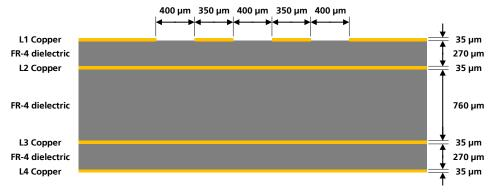
Figure 36: Example of USB line design, with Z<sub>o</sub> close to 90  $\Omega$  and Z<sub>cm</sub> close to 30  $\Omega$ , for the described 4-layer board layup
