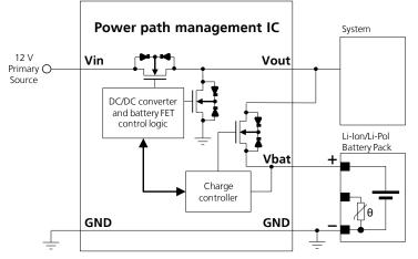
Figure 15: Charger / regulator with integrated power path management circuit block diagram
