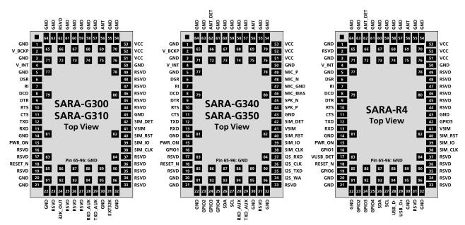
Figure 44: SARA-G3 series and SARA-R4 series and modules pad layout and pin assignment
