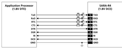
Figure 27: UART interface application circuit with complete V.24 link in DTE/DCE serial communication (1.8V DTE)
