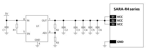
Figure 12: Example of high reliability VCC supply application circuit using an LDO linear regulator
