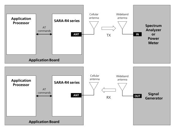
Figure 43: Setup with spectrum analyzer or power meter and signal generator for radiated measurements
