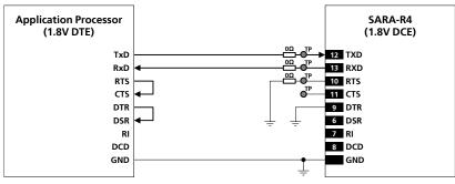
Figure 33: UART interface application circuit with partial V.24 link (3-wire) in the DTE/DCE serial communication (1.8V DTE)
