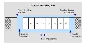
Figure 8: Description of UART 8N1 frame format (8 data bits, no parity, 1 stop bit)
