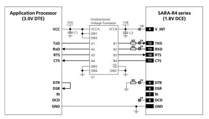
Figure 32: UART interface application circuit with partial V.24 link (5-wire) in DTE/DCE serial communication (3.0 V DTE)
