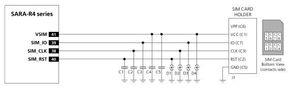
Figure 24: Application circuits for the connection to a single removable SIM card, with SIM detection not implemented
