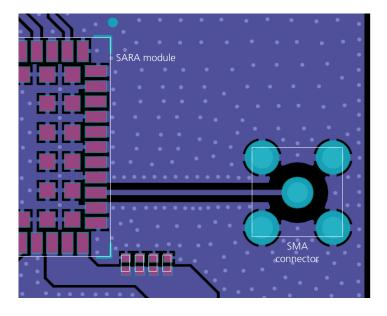
Figure 22: Example of circuit and layout for antenna RF circuits on application board
