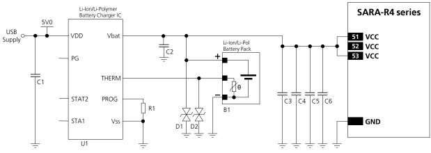
Figure 14: Li-Ion (or Li-Polymer) battery charging application circuit
