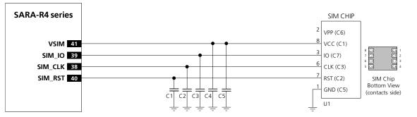
Figure 25: Application circuits for the connection to a single solderable SIM chip, with SIM detection not implemented
