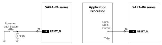
Figure 18: RESET\_N application circuits using a push button and an open drain output of an application processor
