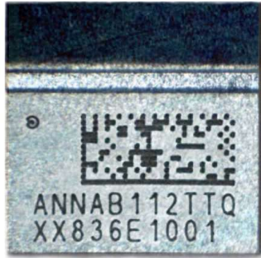
Figure 10: Product marking on the ANNA-B112 module
