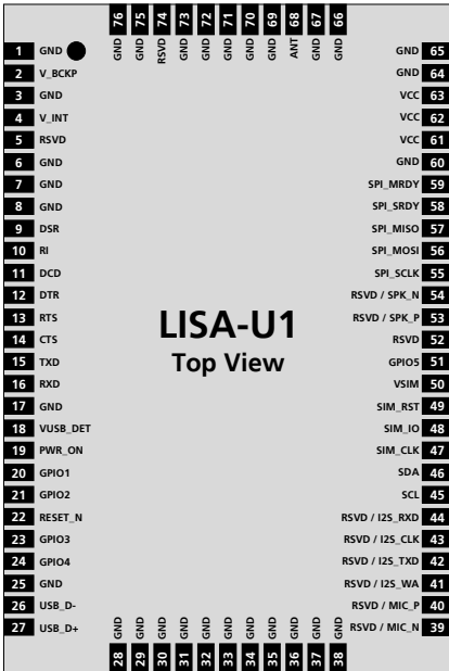
Figure 75: LISA-U1 series pin assignment
