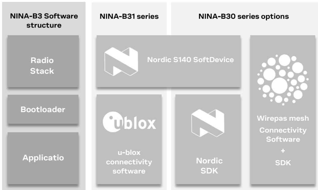
Figure 2: NINA-B3 software structure and available software options
