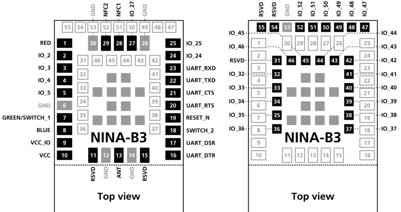
Figure 4: NINA-B31 series pin assignment (top view)
