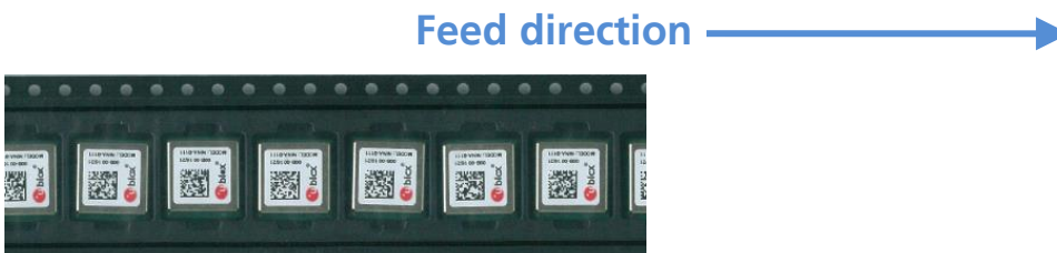
Figure 9: Orientation of NINA-W101 module on tape
