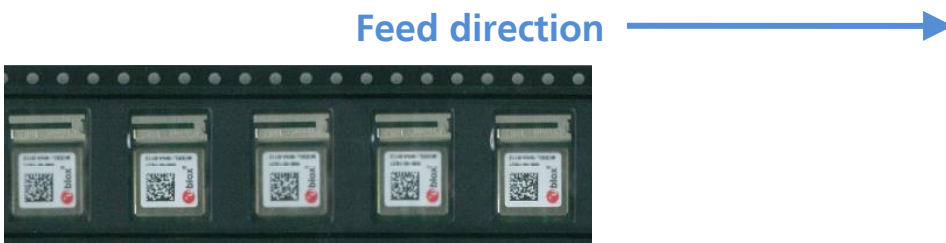
Figure 10: Orientation of NINA-W102 module on tape
