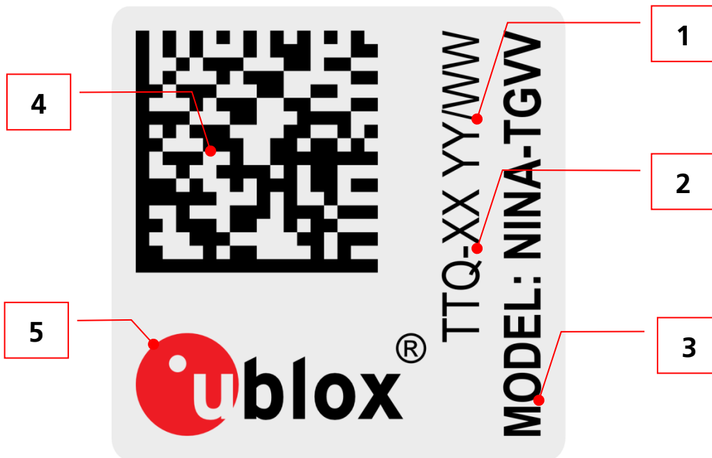
Figure 12: Location of product type number on the NINA-W13 series module label
