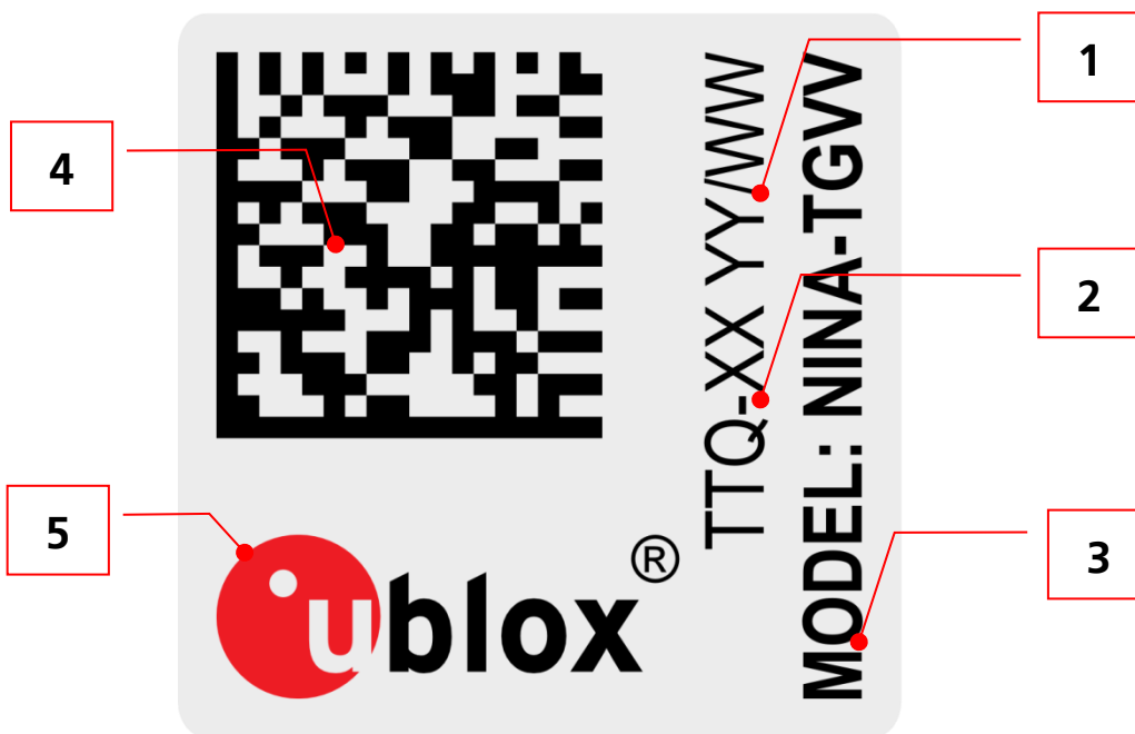
Figure 13: Location of product type number on the NINA-W15 series module label
