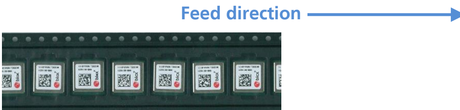
Figure 9: Orientation of NINA-W151 module on tape
