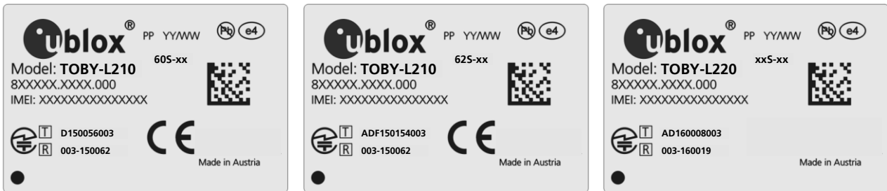
Figure 78: Label of TOBY-L210-60S, TOBY-L210-62S and TOBY-L220 modules product versions with Giteki mark
