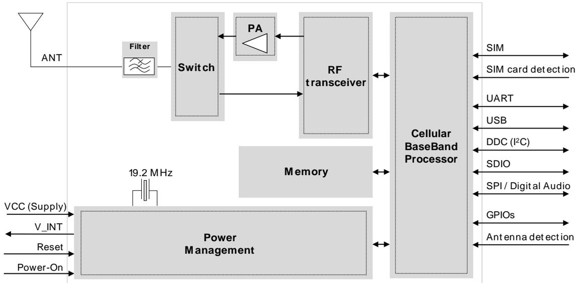
Figure 1: SARA-R4/N4 series modules simplified block diagram
