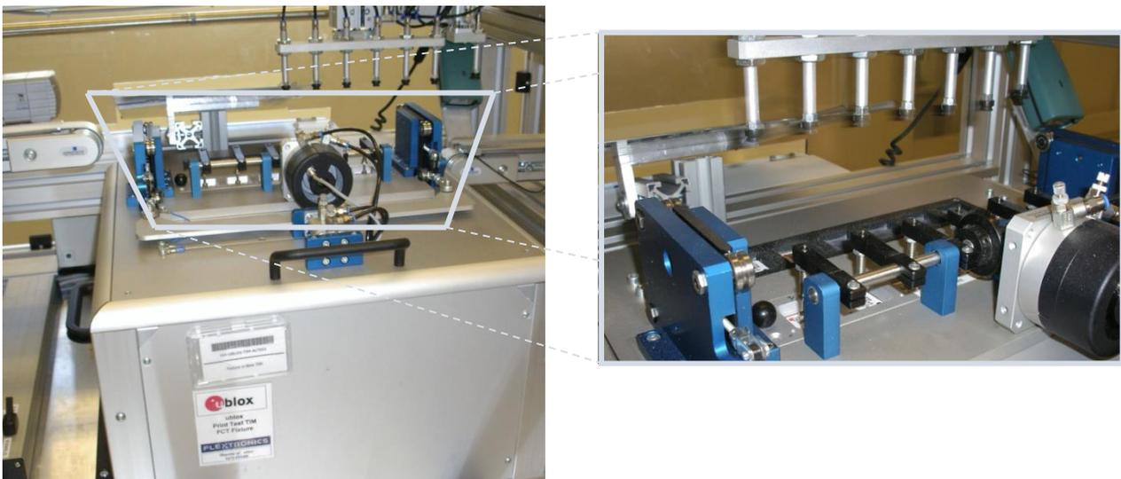
Figure 57: Automatic test equipment for module tests
