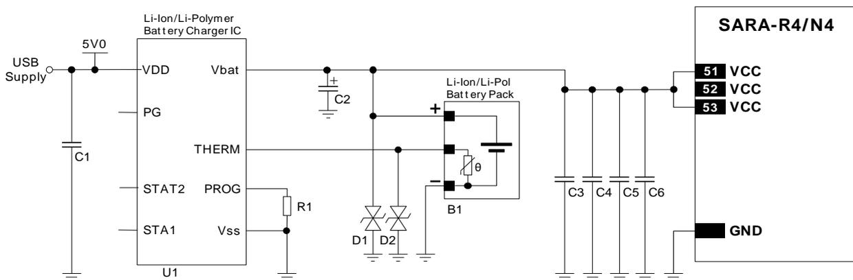
**Figure 22: Li-Ion (or Li-Polymer) battery charging application circuit**
