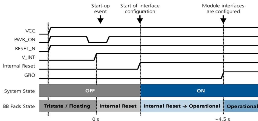
Figure 9: SARA-R4/N4 series switch-on sequence description
