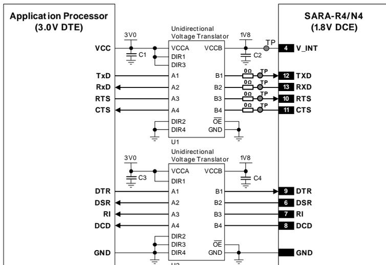
Figure 41: UART interface application circuit with complete V.24 link in DTE/DCE serial communication (3.0 V DTE)
