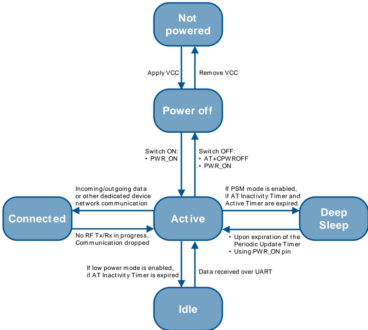
Figure 2: SARA-R4/N4 series modules operating modes transitions
