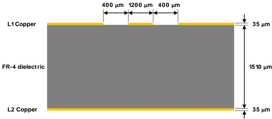
**Figure 33: Example of 50 Ω coplanar waveguide transmission line design for the described 2-layer board layout**
