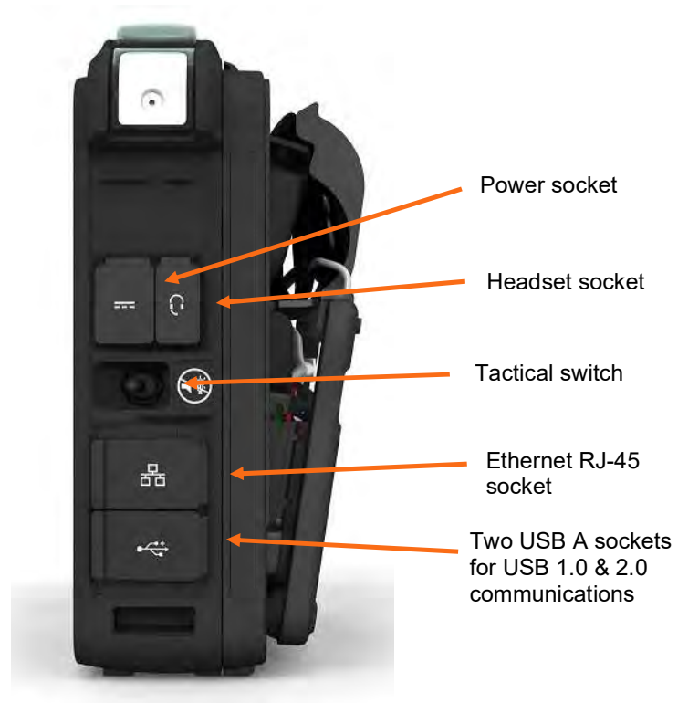
Right Side of the Tempus – Communications Connectors
