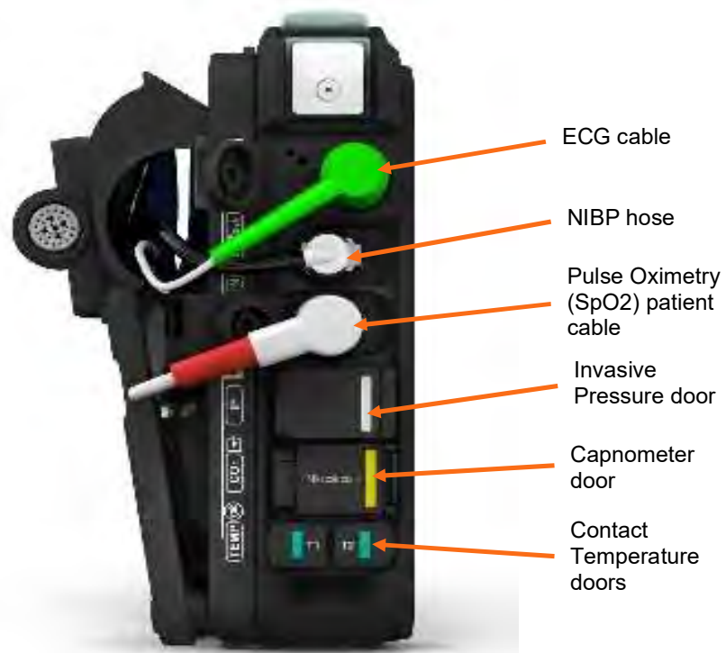
Left side of the Tempus – medical connectors
