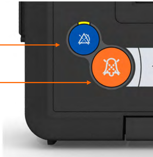
Alarm Suspend and Silence Buttons
