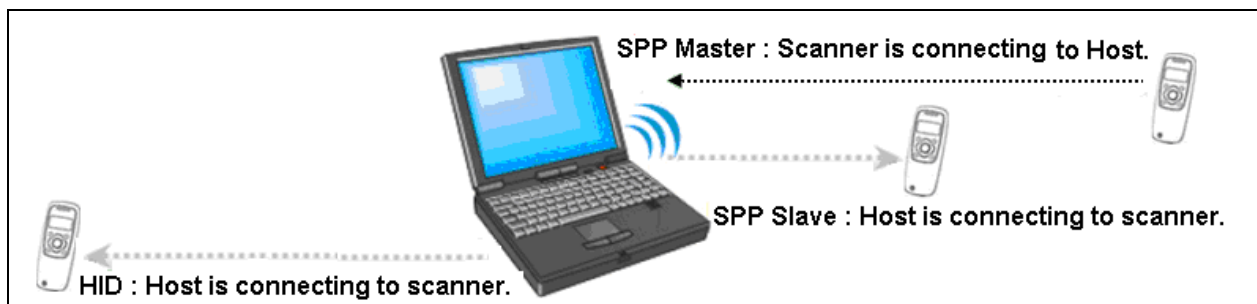
Figure 5-1. Diagram of Bluetooth functionalities
