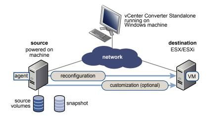
4 Optionally, Converter Standalone uninstalls the agent from the source machine.The virtual machine is ready to run on the destination server.
