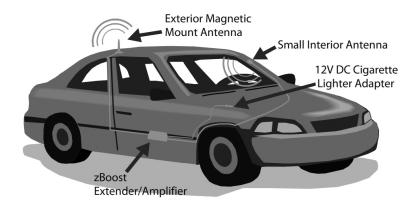
The above diagram is one example of a recommended installation. Other variations are possible. Consult your local mobile electronics installer.
